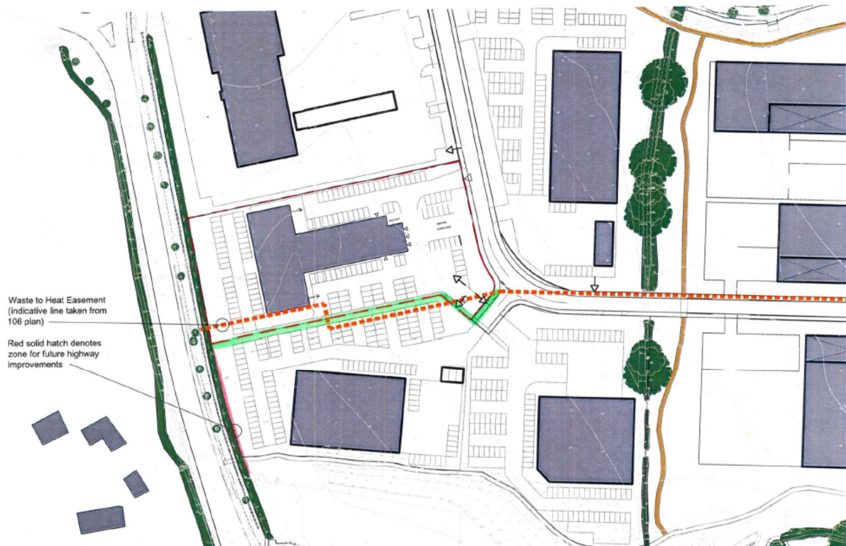
Figure 6-2: Pipe easement through Matford Park
