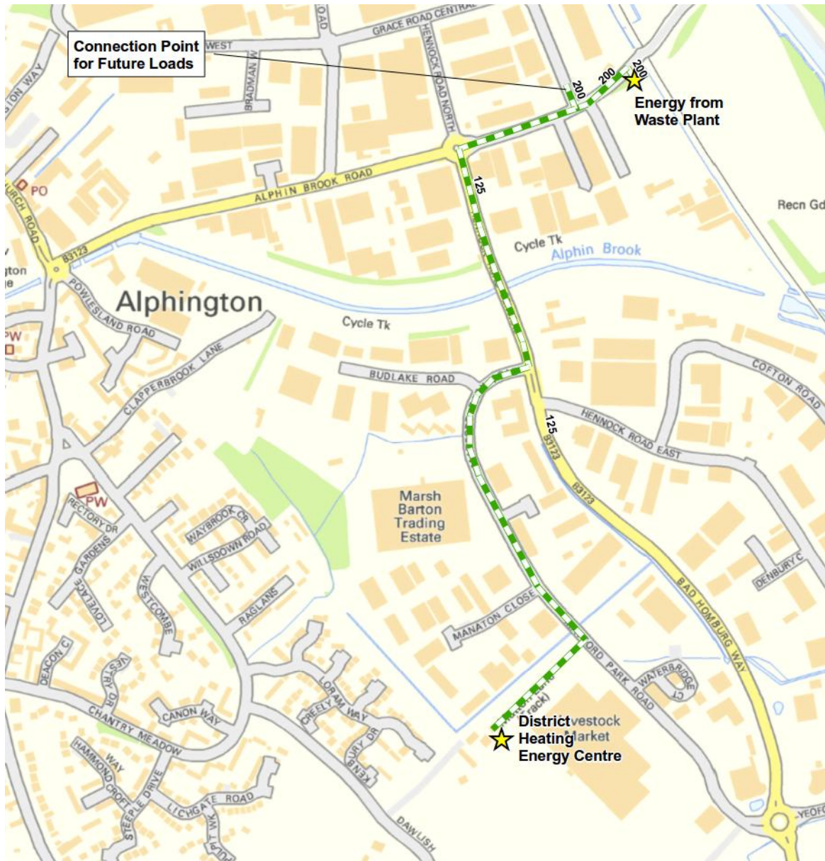
Figure 6-5: Transmission main alternative route
